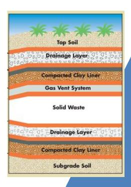
Vegetative Cover – reduces infiltration, wind erosion, and improves slope stability.
